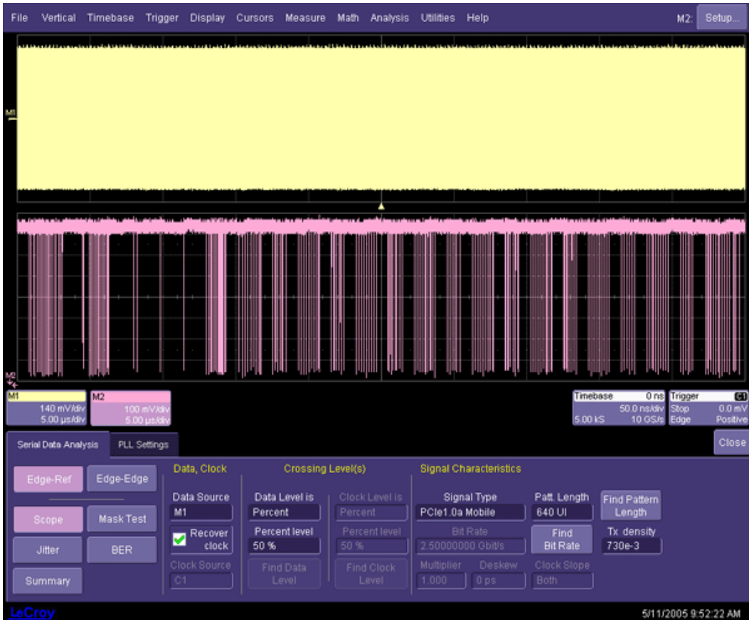
Data (M1) and Gate (M2) signal sources
