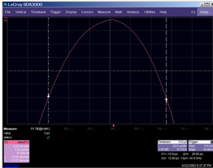
Figure 9. Total jitter curve. The vertical values of this curve represent the probability of a data transition occurring at a time represented by the horizontal axis. The horizontal center of the plot is 0 ps. The two markers are placed at the vertical level corresponding to a bit error rate of 10^{-12} and the horizontal distance between these two points is the total jitter at this bit error rate.
